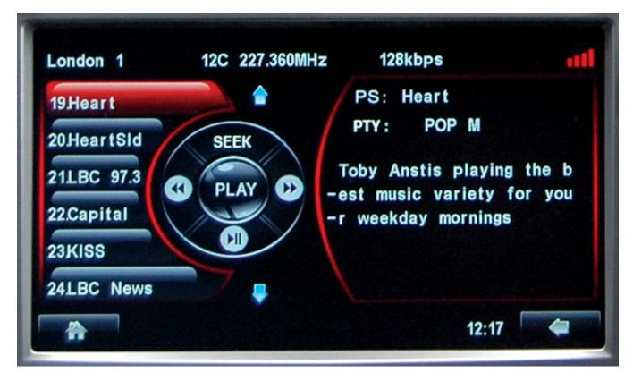
4. Once tuned in, the stations will show in a list on the left-hand side of the screen, with the station information on the right-hand side.
